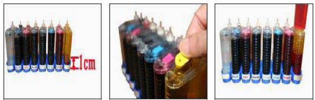
Please pay attention to the ink level in the reservoirs; if the ink level is below 1CM as the above picture shown, please use refill kits to fill ink into Reservoir bottles. Carefully pull out the rubber plugs from the refill holes. (There is possibility of ink spattering. Be careful!) Refill ink according to the color in short supply. Then put the rubber back. (Please keep the printer and the reservoir at the same horizontal line during the process of refilling ink.)
