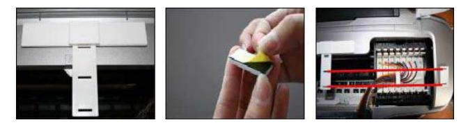
Fix the balance arm stick on the support arm as show on the picture, Rip the label on the shortest arm, And Stick it on the right side of the printer, but need to keep it in the same horizontal line as show in the picture.
