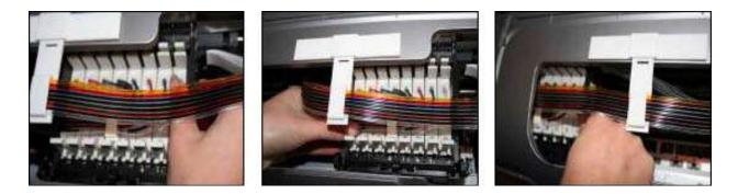
Adjust the tube length and move the cartridge car. Insure there will no block and collision when the tubes moving with cartridge car .Insure there's plenty length of tube to make the cartridge cart can thoroughly move to the right side.
