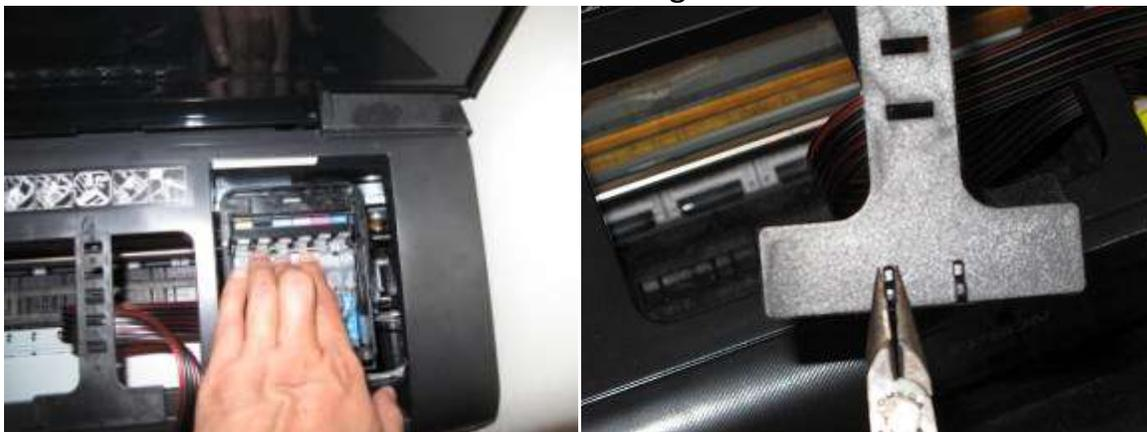
4. The fourth step: Fix up the support arm and install the tubes
