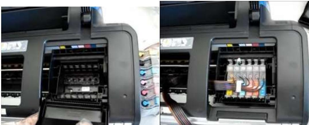
3. Place down each cartridge according to the color, in the meantime; make every cartridge in the correct position by press down the cartridge until you hear the “click” sound for each cartridge.
