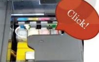
Looking into the printer from above, install the support clip(s) as shown. The one on the left (in the photos below) is called a *square clip*.
