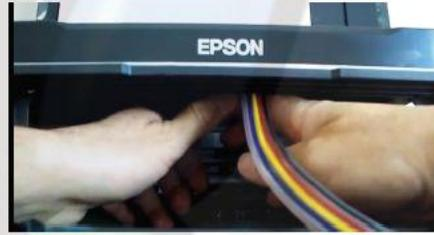
After you have attached the pipeline with the clip(s) check that it has enough slack so that the printer head can move through its entire range without stretching the pipeline or potentially blocking it.
