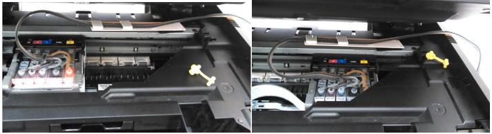
Install the switch jumper on the right side as shown. This will stop the lid from closing too far. Feed the hose out of the printer and close down the lid. The lid will not be completed closed.
