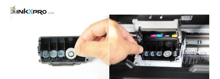
Remove orange cartridge caps and install cartridges. After removing orange cartridge caps make sure to keep cartridges above the ink reservoirs and install cartridges quickly. Because ink may leak from the cartridges once the orange plugs are removed. Have some paper towels ready in case any ink drips.
