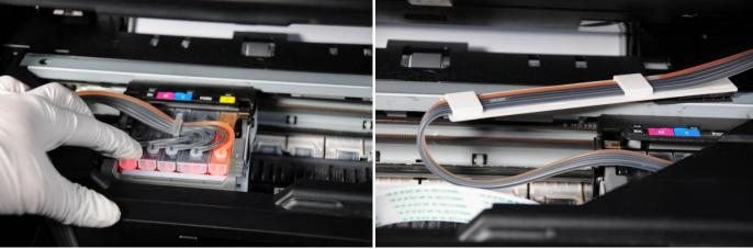
Now peel and attach bracket with the ink tube as pictures above showed. Move the cartridge to right side and left side; adjust the length of the tube.
