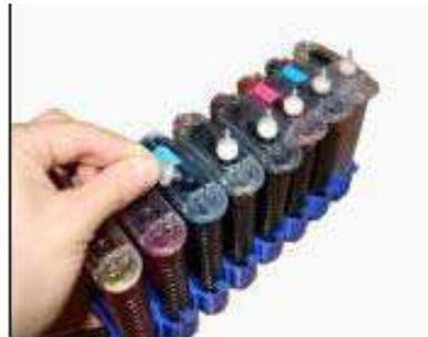
Put the CISS on the right side of the printer. In the meantime place all the tubes at correct position.
