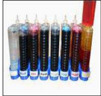
Please pay attention to the ink level in the reservoirs; if the ink level is below 1CM as the above picture shown, please use refill kits to fill ink into Reservoir bottles. Carefully pull out the rubber plugs from the refill holes. (There is possibility of ink spattering. Be careful!) Refill ink according to the color in short supply. Then put the rubber back. **(Please keep the printer and the reservoir at the same horizontal line during the process of refilling ink.)**
