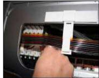
Adjust the tube length and move the cartridge car. Insure there will no block and collision when the tubes moving with cartridge car .Insure there's plenty length of tube to make the cartridge cart can thoroughly move to the right side.
