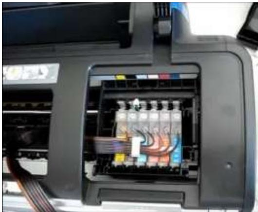
3. Remove out the original cartridges, then place down each cartridge according to the color, in the meantime, make every cartridge in the correct position.
